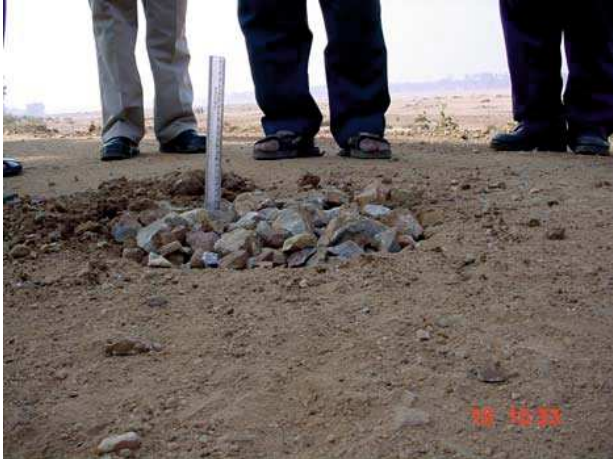
Photographs showing plastic Crushable aggregate used in WBM but good compaction
