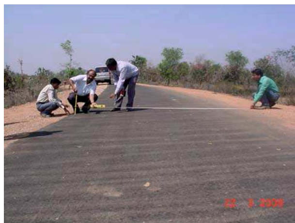
Photographs showing measurements of carriage way width, camber and super-elevation.
