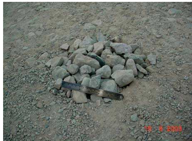
Photographs showing plastic Crushable aggregate used in WBM but good compaction
